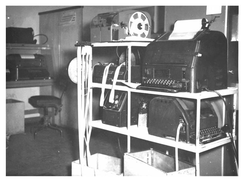
This assembly consisting of T-Lock 15 monitor, transmit distributer, page printer, sequence control unit and reperforator is used in conjunction with the KW-26 crypto consoles to provide continuous secure communications 24 hours per day with DSD.
