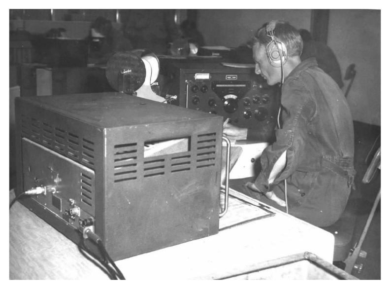
This picture shows the layout of a handspeed morse position which is equipped with 2 Collins 51-J4 receivers, a typewriter, aerial selectors capable of selecting any one of eleven aerials, set selector and headphones.
