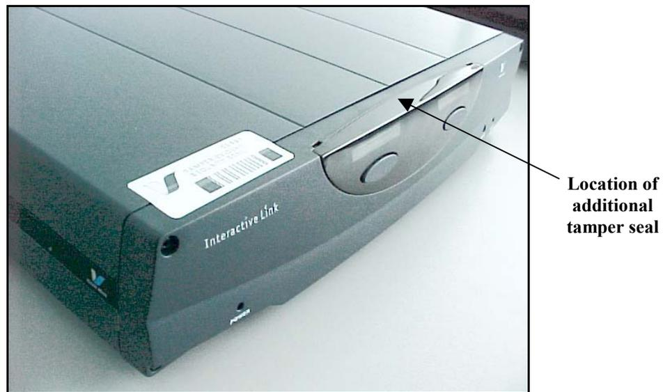
**Figure 1 - Additional Tamper Seal Location for High Security Environments**
