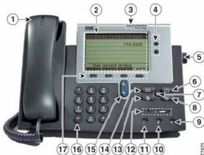
Figure 2: Front View of the Cisco IP Phone 7960G
